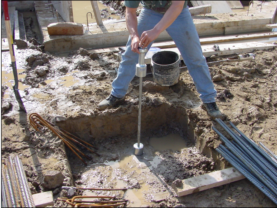
Photo 7. Undisturbed sampling of stiff stratum in north Amherst, NY.
