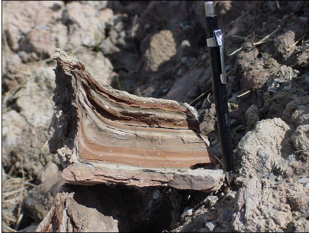
Photo 1. Varved clay from excavation near Millersport and Transit Roads. Sample characteristic of lacustrine material in Lake Dana-Lundy (D'Agostino, 1958). Laminated bands thought to indicate annual cycles of deposition from summer (pink) to winter (gray).
