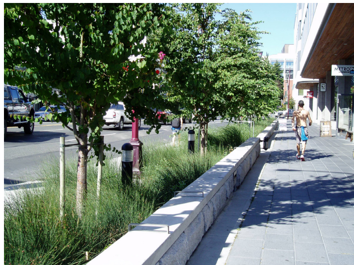
This curb zone incorporates seating, pedestrian-level lighting, shading trees and stormwater retention landscaping.
