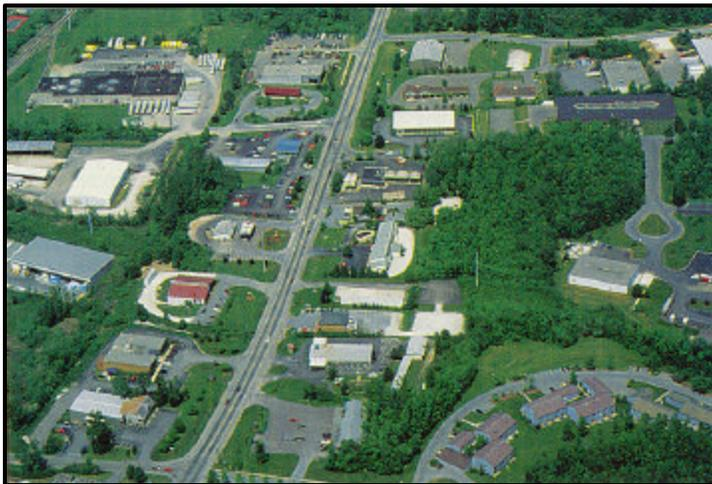
Figure 5-4 Highway commercial designed as typical suburban strip with no access management provisions
